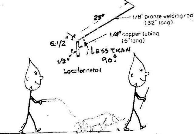
Some persons can locate pipe by the use of a pair of bronze rods held as shown in this drawing of an underground pipe locator. When the rods pass over a buried pipe, they swing apart.
